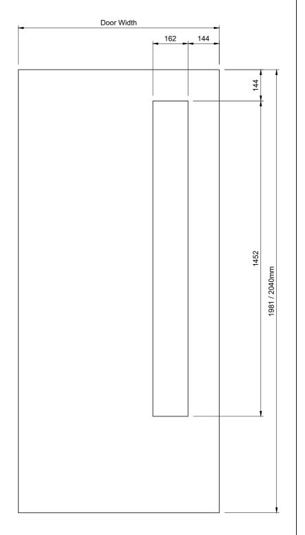
Description Doorpac Standard Aperture - 20G - 150 x 1440mm - 150mm Top & Side Margins - FD60 Machining
